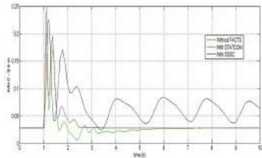
Figure 10. Delta between generator 1 and 2
