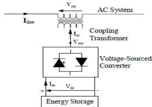
Figure 2. Functional model of SSSC
