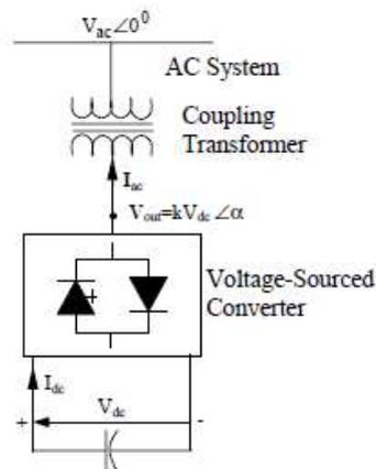
Figure 1. Functional model of a STATCOM
