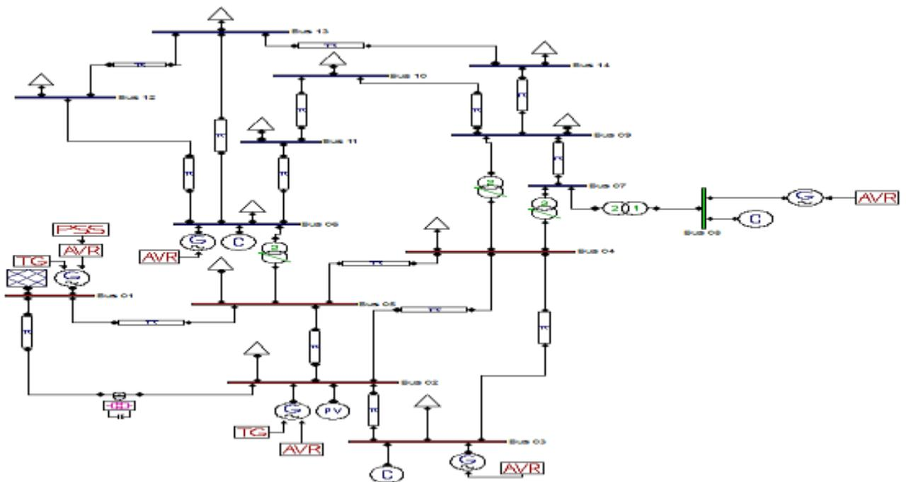
Figure 3. IEEE 14-bus system with (SSSC) Simulation model in PSAT/Simulink.
