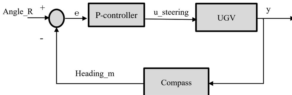
Figure 6. Closed-loop control of the system
