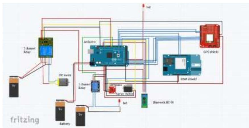
Figure 3. Full circuit of the proposed system
