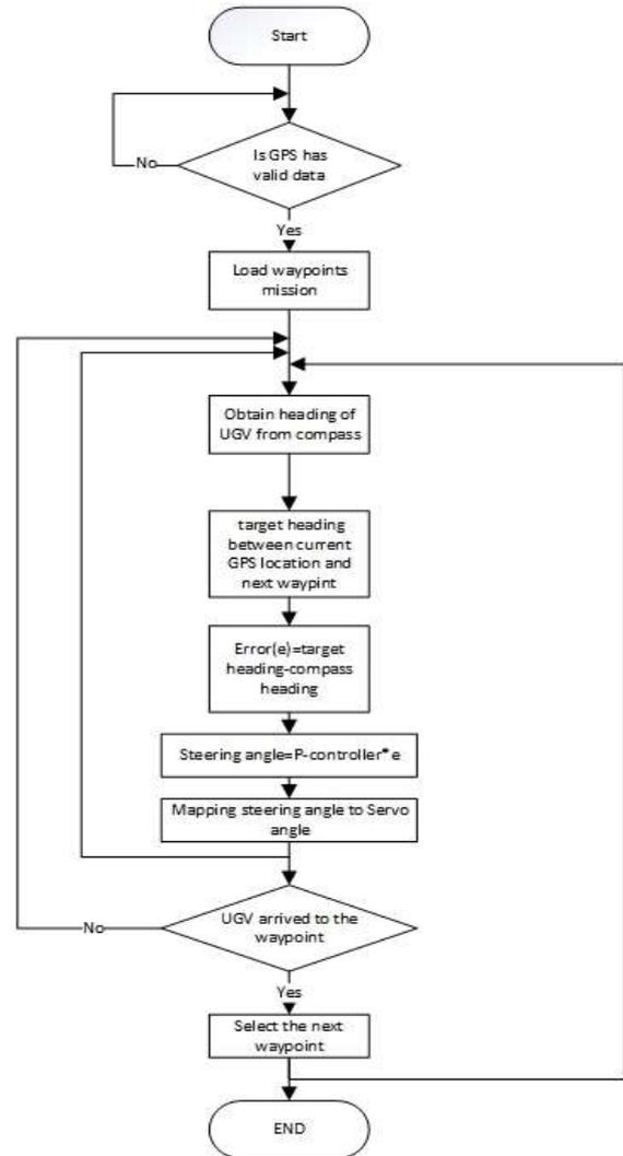
Figure 5. Autonomous mode of the UGV
