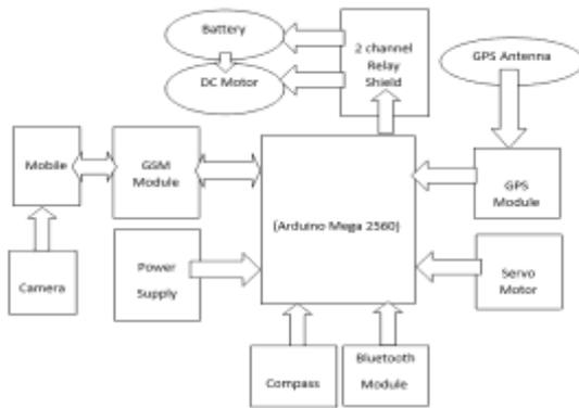
Figure 1. Block diagram of UGV
