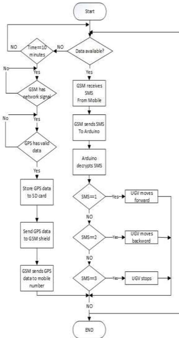
Figure 4. Manual mode of the UGV
