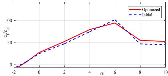
Figure (7) Comparison of L/D ratio
