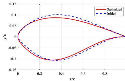
Figure (8) Comparison between initial and optimum airfoil shapes
