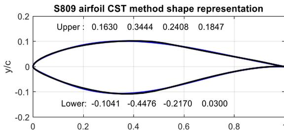
Figure 1 Representation of S809 airfoil with 4 parameter CST method
