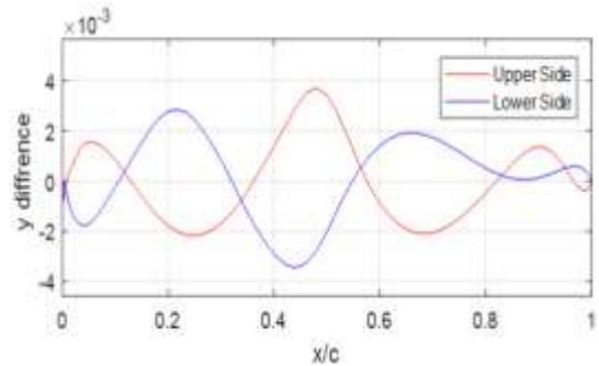
Figure 2 Difference in airfoil y coordinates between original and CST representation
