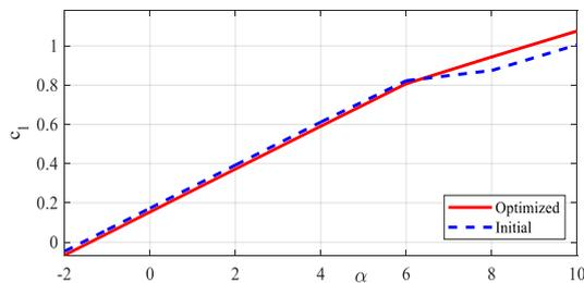
Figure (6) Variation of lift coefficient with angle of attack
