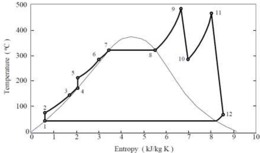
Figure 2. Temperature-entropy diagram of Rankine cycle
