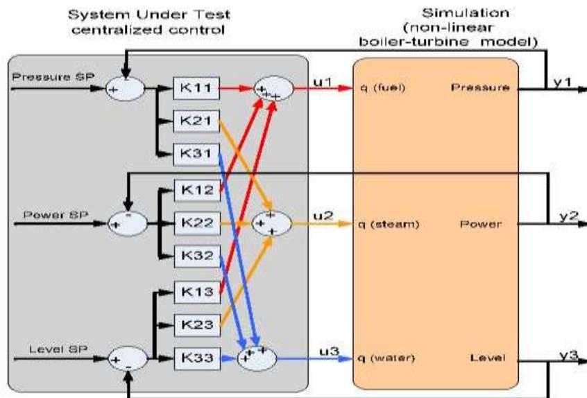
Fig 3 . Centralized control using a unity feedback control structure
