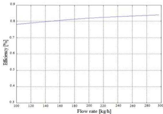
Figure 7 Effect of water flow rate on the solar collector thermal efficiency
