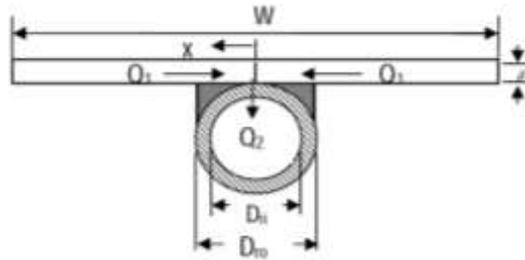
Figure 1 Fin and tube section
