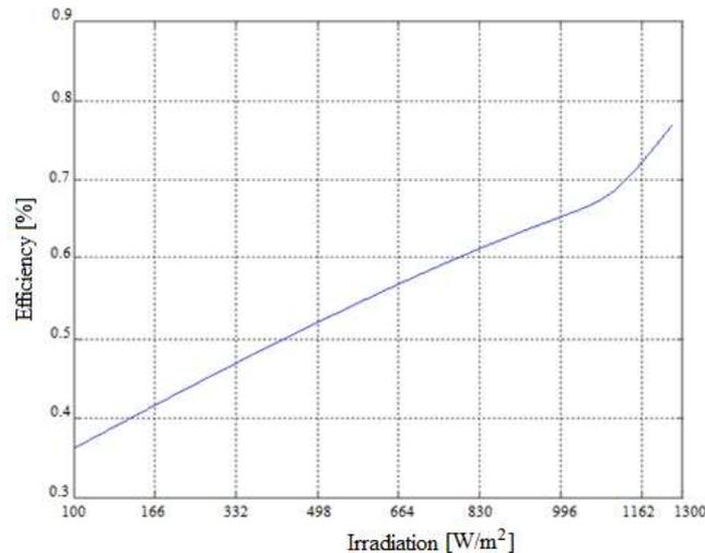
Figure 10 The influence of irradiation on the collector thermal efficiency
