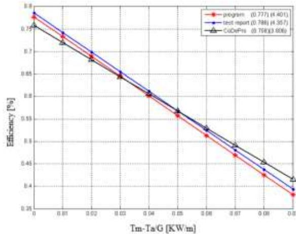
Figure 5 Comparison between one and two dimensional algorithm results and the tested collector.
