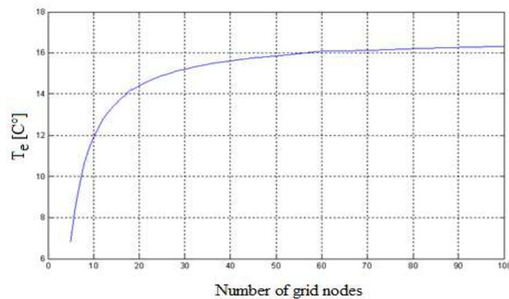
Figure 3 The influence of the grid on the outlet temperature.
