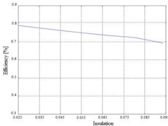
Figure 6 Effect of insulation on the solar collector thermal efficiency.
