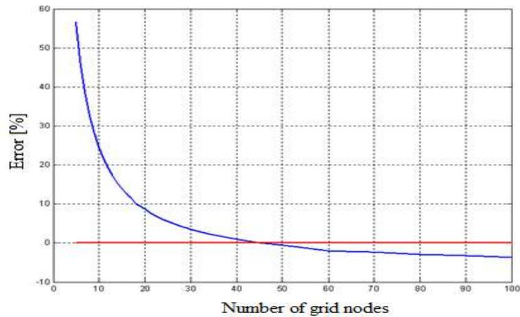
Figure 2 Algorithms error in function of mesh grid.
