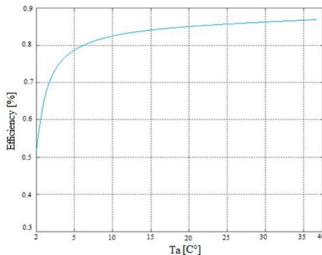
Figure 9 Effect of ambient temperature on the collector thermal efficiency.
