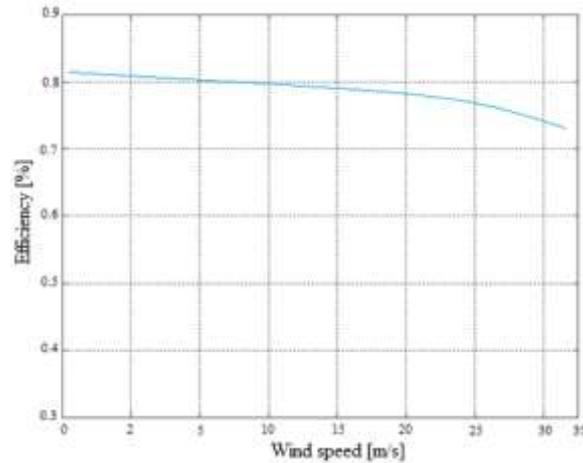
Figure 8 Influence of wind speed on the solar collector thermal performance
