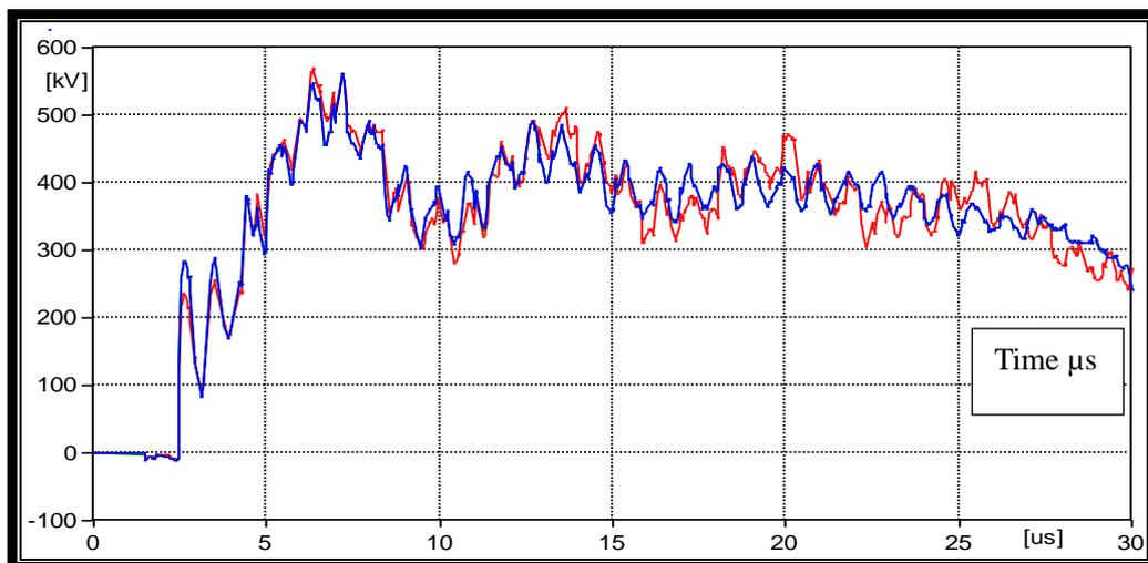
Figure7. The inside voltage of the transformer at  $R_{\text{foot}} 10\Omega$  by current 150KA
