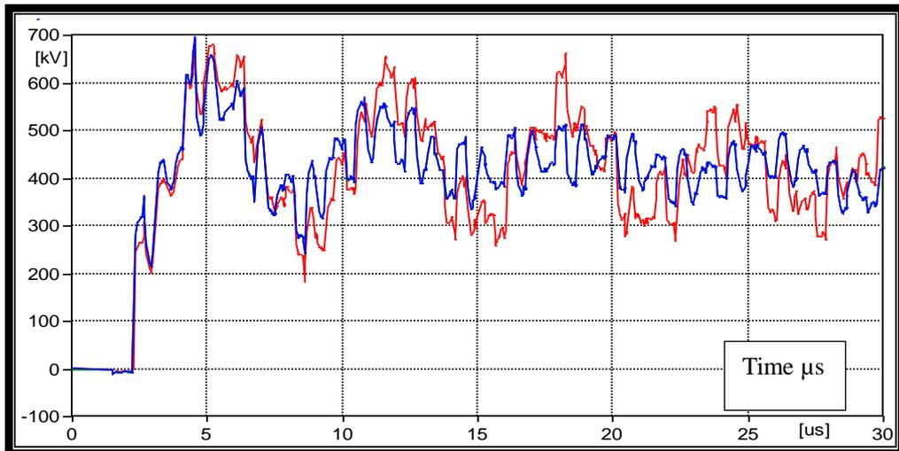
Figure 4. The inside voltage of the transformer at  $R_{foot} 25\Omega$  by current 150KA
