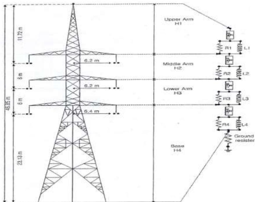
Figure 2. 220kV Tower configuration
