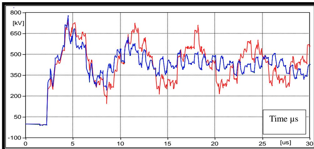
Figure 5. The inside voltage of the transformer at  $R_{foot} 35\Omega$  by current 150KA
