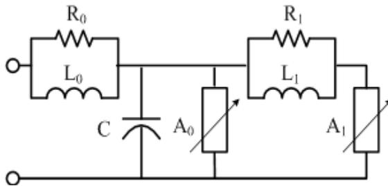
Figure 3. Model of MO arrester according to IEEE standards.
