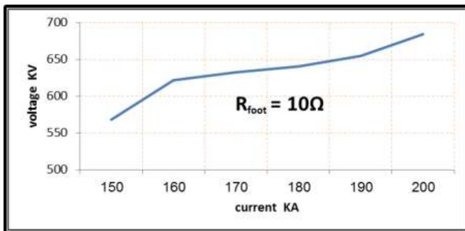
Figure 8. Effect of the lightning currents on inside voltage for transformer at R<sub>foot</sub>(10Ω)
