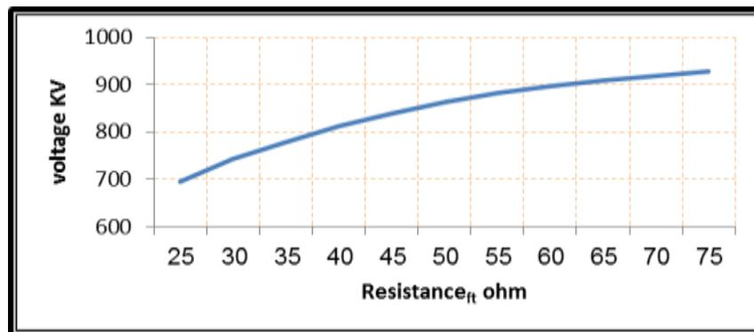
Figure 6. Effect of the tower footing resistance on inside voltage of transformer when be 150KA lightning current.
