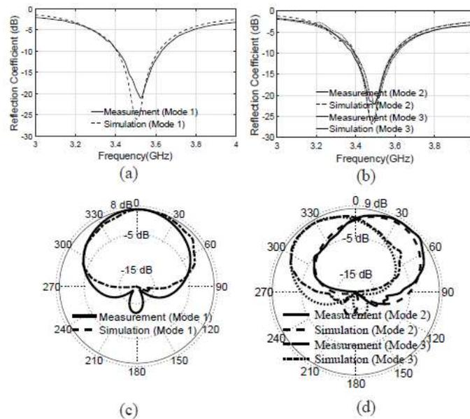
Fig. 2: Simulated and measured reflection coefficients of the RA for (a) mode 1 and (b) modes 2,3, and realized gain patterns for (c) mode 1 and (d) modes 2,3
