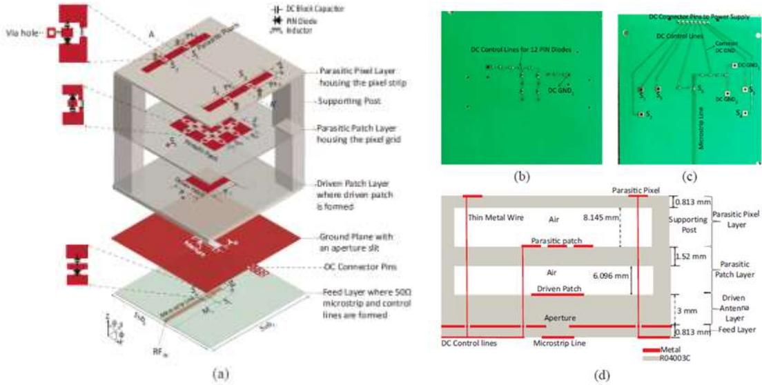
Fig. 1: (a) 3D exploded view of the RA, photograph of bottom face of the (b) parasitic patch layer and (c) feed layer, and (d) AA' plane cross section of the RA.
