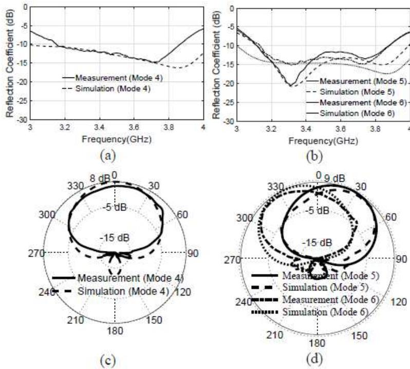
Fig. 3: Simulated and measured reflection coefficients of the RA for
