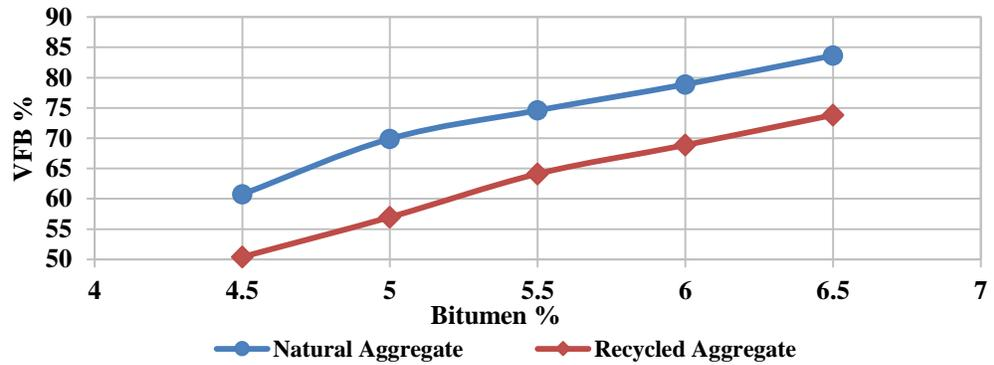
Figure 5: Voids filled bitumen proportion vs bitumen content
