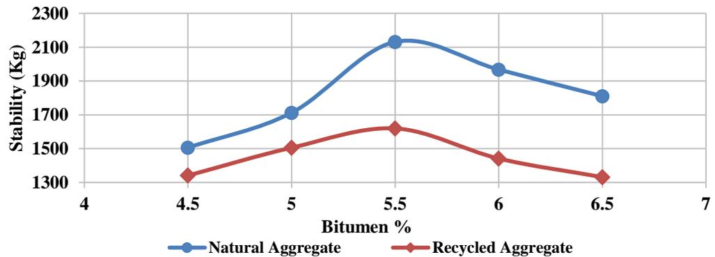
Figure 6: Stability vs bitumen content
