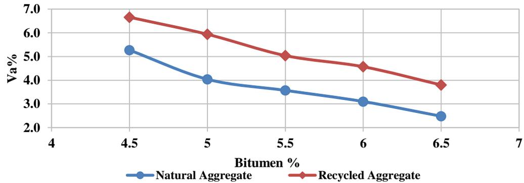
Figure 3: Air voids proportion vs bitumen content
