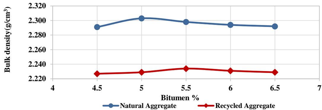
Figure 2: Bulk density vs bitumen content
