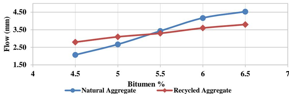
Figure7: Flow vs bitumen content
