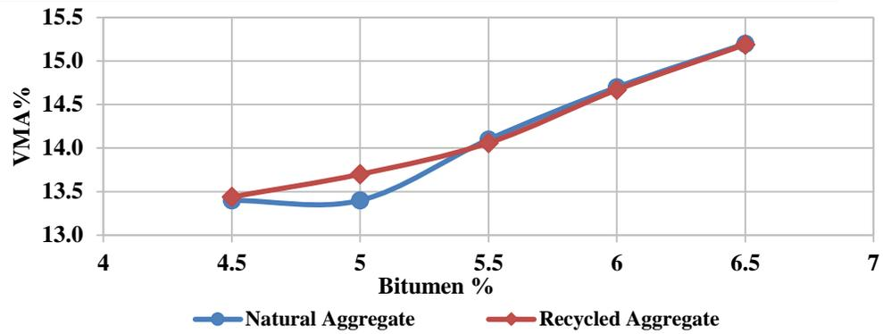
Figure 4: Voids of mineral aggregate proportion vs bitumen content
