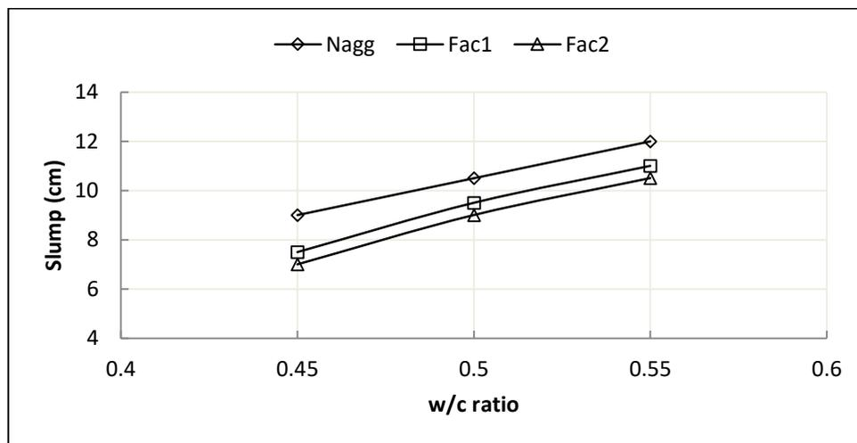
Figure 1 Relation between slump and w/c ratio
