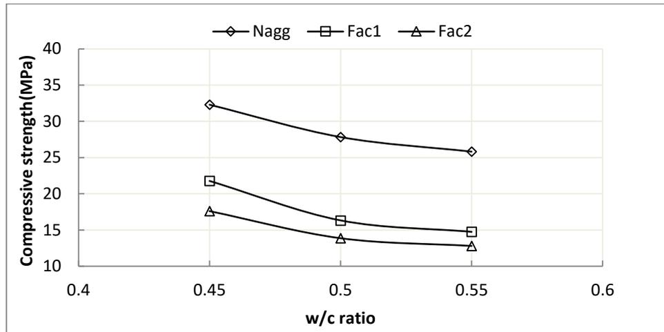
Figure 2 Relation compressive strength and w/c ratio
