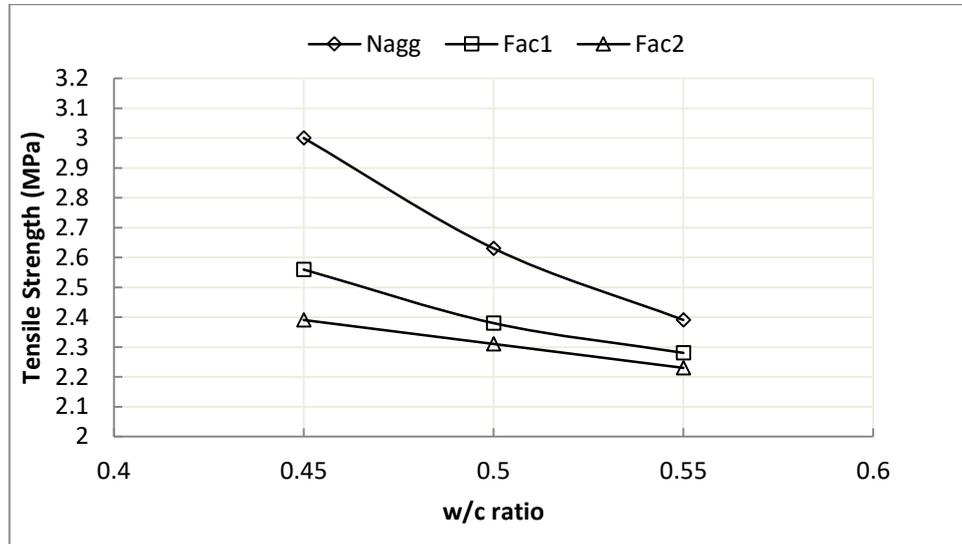
Figure 3. Relation between tensile strength and w/c ratio
