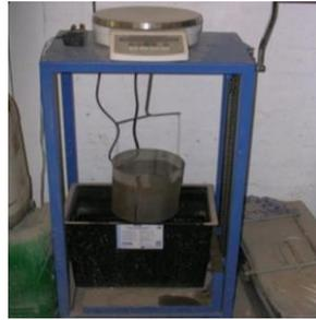
Fig. 5. Density testing apparatus (weight-in-air/weight-in-water method)
