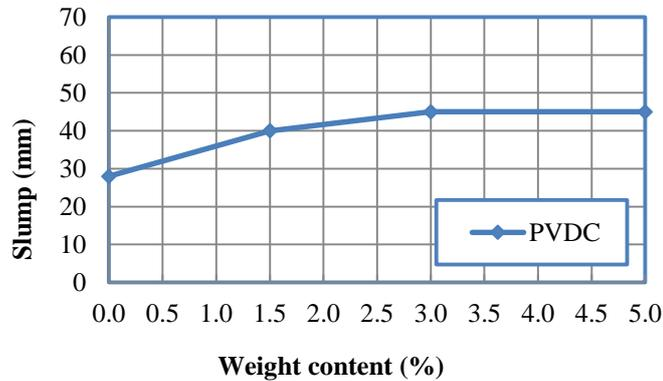
Fig. 9. Measured slump values for the HPC with different contents of PVDC
