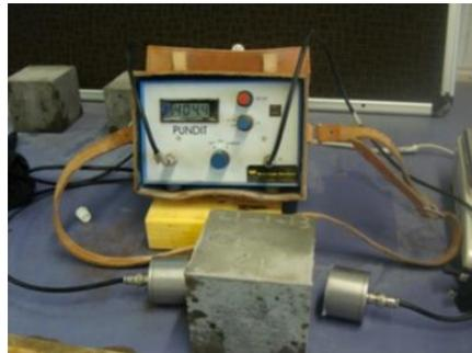
Fig. 8. Pundit ultrasonic tester for measuring the dynamic elastic modulus
