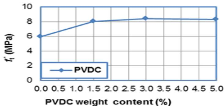
Fig. 13. Splitting tensile strength of the HPC with different contents of PVDC at 28 days
