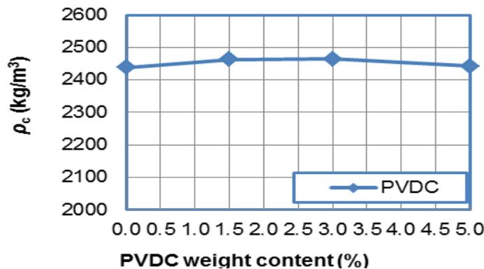
Fig. 10. Densities of the HPC with different contents of PVDC at 28 days
