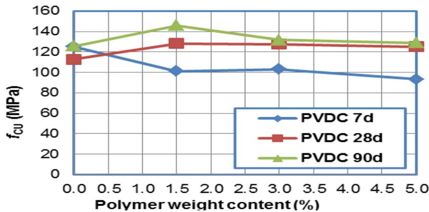
Fig. 12. Compressive strength of the HPC with different contents of PVDC at 7, 28 and 90 days
