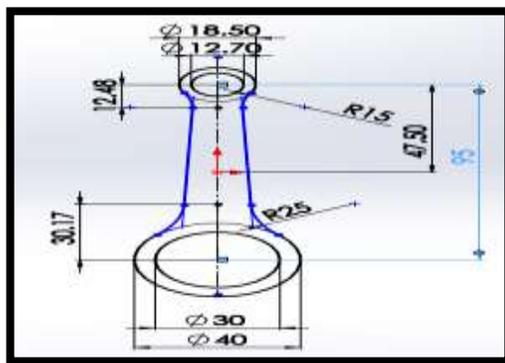
Figure 1 The base sketch of the connecting rod
