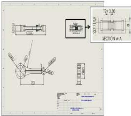
Figure 8 Drawing of the connecting rod showing few of the dimensions that are design variables and dimensions that cannot be changed
