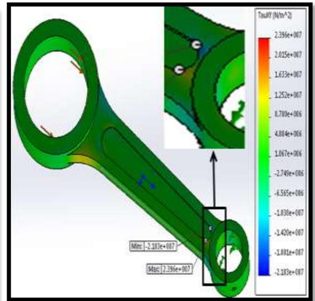
Figure 4 Shear stress distribution with static compressive load of 4319 N at the crank end
