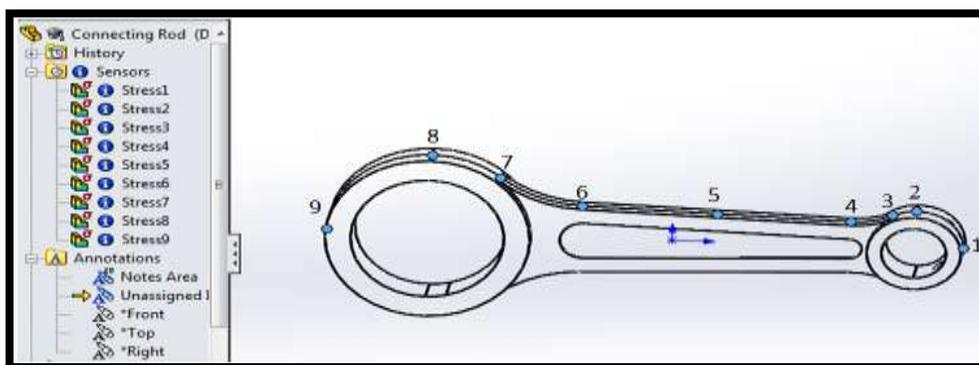
Figure 4 sensors to record Von Mises stress data at a few discrete locations on the mid plane labeled on the connecting rod, along the length
