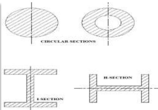
Figure 2 Schematic illustration of types of cross sectional
