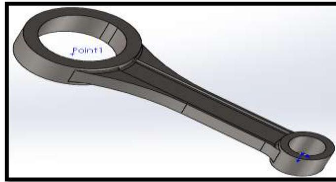
Figure 10 The geometry of the optimized connecting rod
