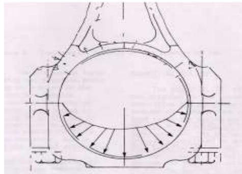
Figure 3 Tensile loading of the connecting rod
