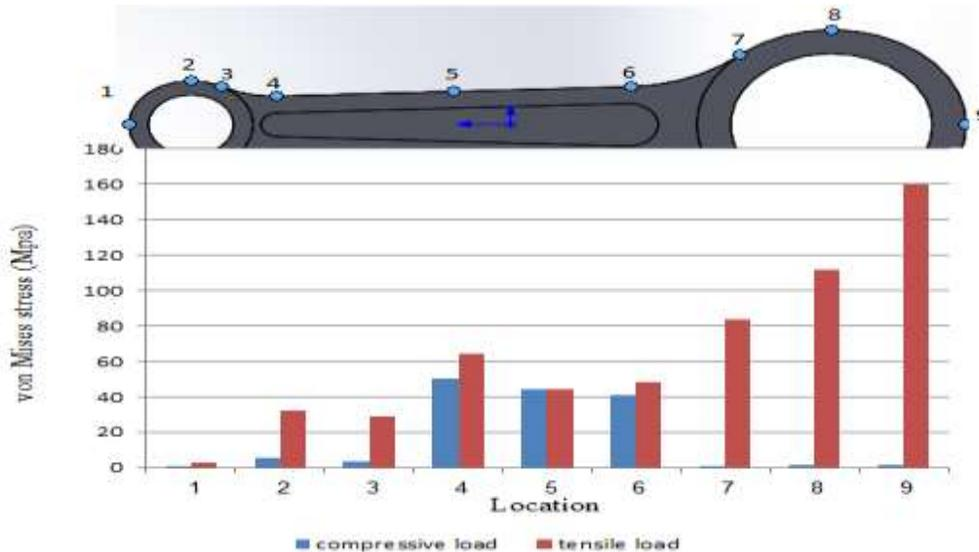
Figure 5 Von Mises stress at a few locations on the mid plane labeled on the connecting rod, along the length, for tensile and compressive loads
