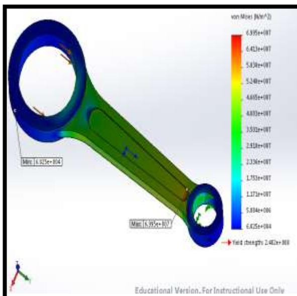
Figure 3 von mises stress distribution with static compressive load of 4319 N at the crank end
