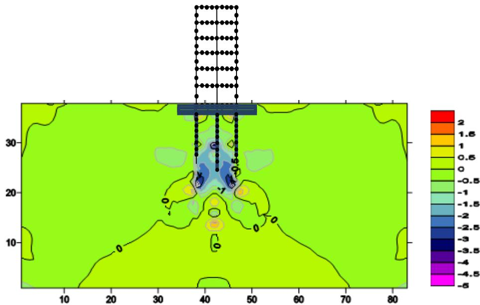
Figure 6 (a): Contour of variation  $\sigma_x$ (First load combination)
