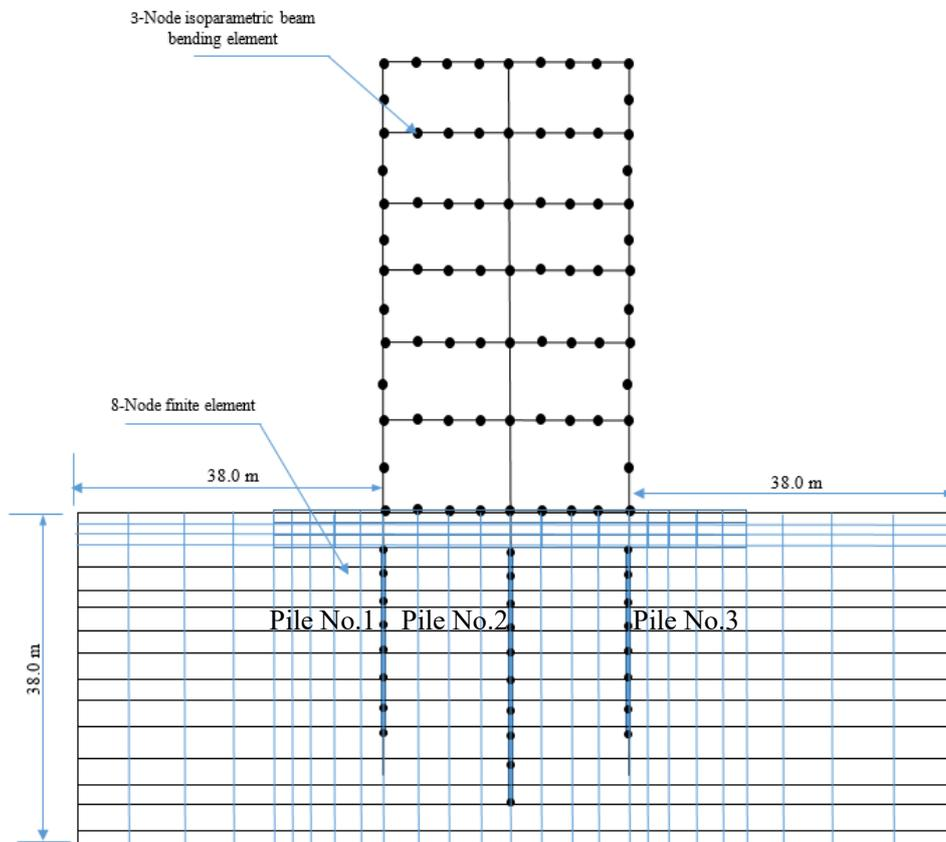
Figure 3. Finite Element Modeling Structure- Mat Foundation- Pile/ Soil
