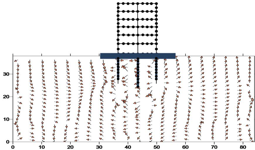
Figure 4(a). Contour of displacement for first load combination (dl+ ll)
