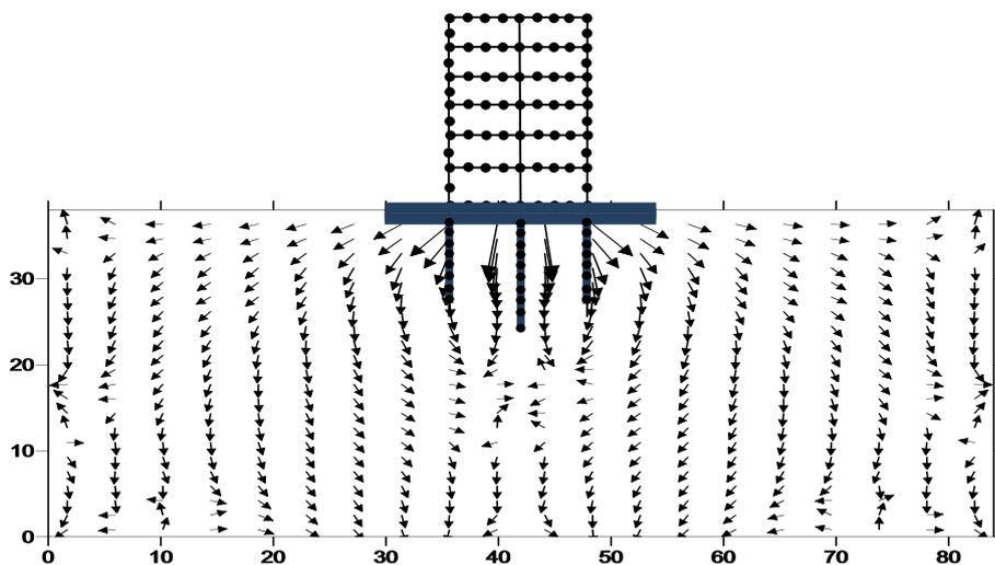
Figure 4(b). Contour of displacement for second load combination (dl+ wind)
