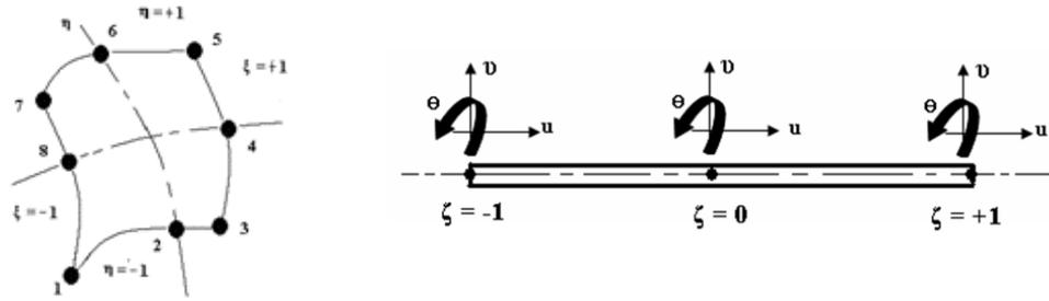
Figure 2. Parabolic isoperimetric Elements
