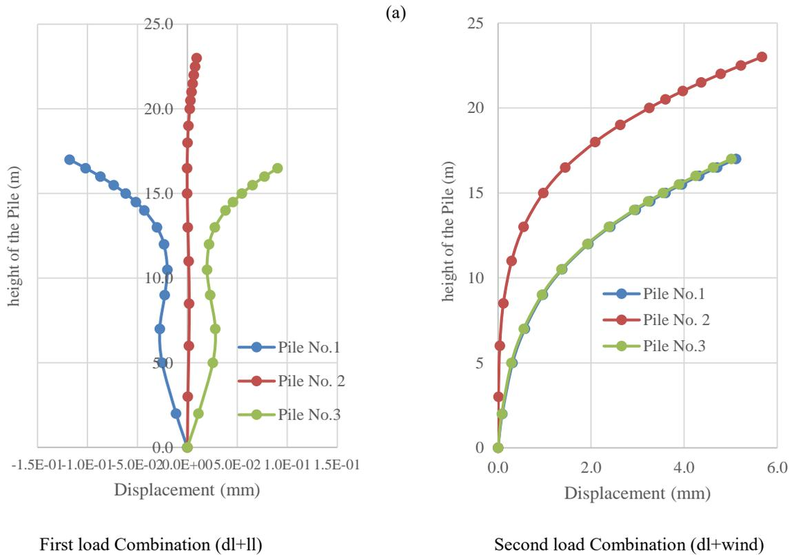
Figure 5. Lateral movement of piles
