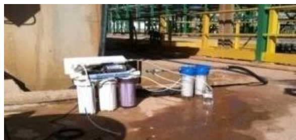
Figure (2) Microfiltration and Single Pass R.O setup used for water desalination.
