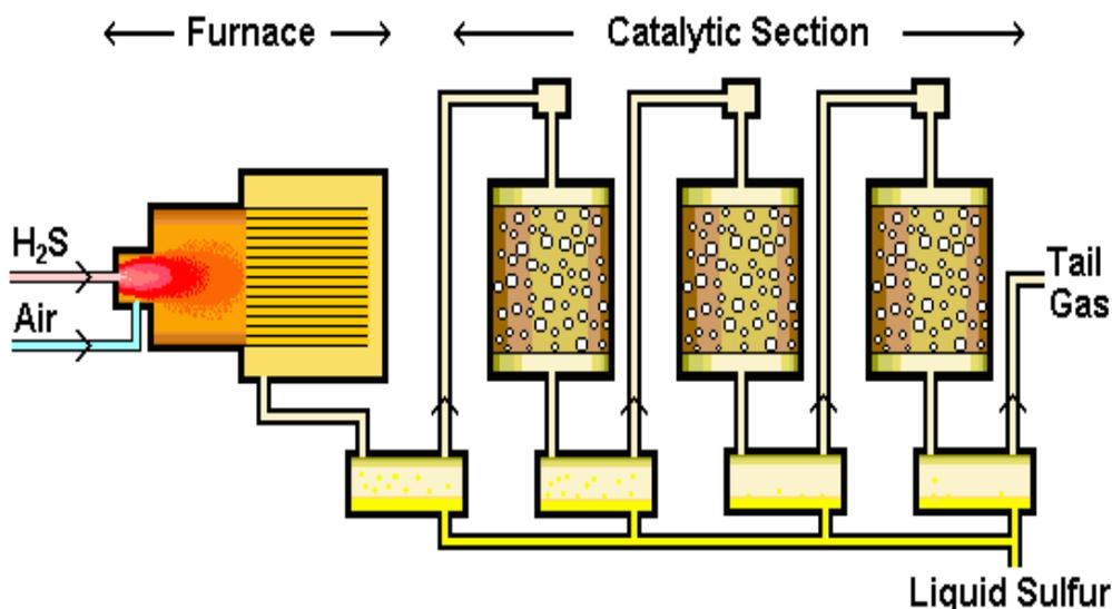
Figure 1: Typical arrangement of a Claus unit
