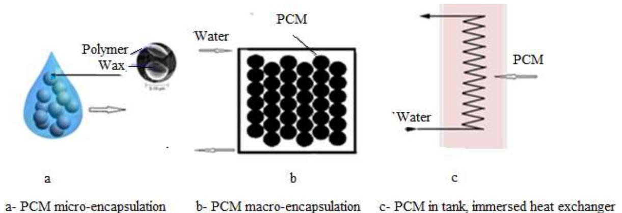
Figure 1.1: Integration of phase change materials into (TES), [2]
