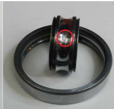
Figure. 5-2 Inner Race Defect
