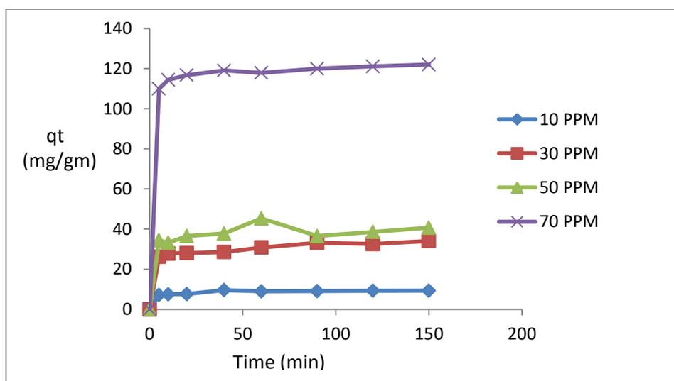
Figure. 6 Effect of initial CR concentration on the amount of adsorption (removal) of CR onto raw pine leaves powder: Mass of Adsorbent: 15 mg; Volume of CR Solution: 50 ml; pH: 6.25; Temperature: 30 C; Shaker Speed: 150 rpm.
