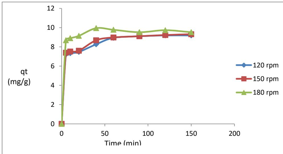
Figure. 7 Effect of agitation speed on the adsorption of CR onto pine leaves; volume of dye solution: 50 ml, initial dye concentration: 10 ppm, temperature: 30 °C, pine leaves dosage: 15 mg, pH: 6.25
