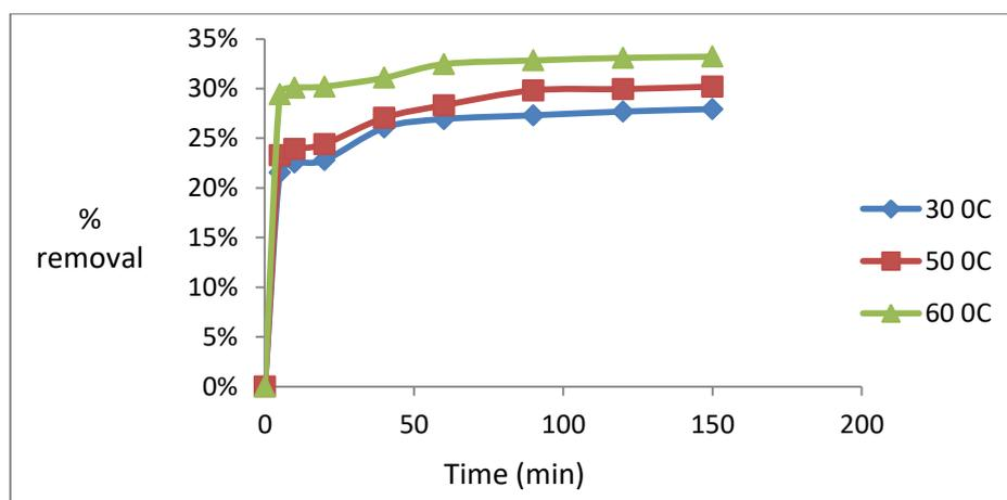
Figure 5 Effect of temperature and time contact on the adsorption of CR onto raw pine leaves powder: Mass of Adsorbent 15 mg; Volume of CR Solution 50 ml; Initial CR Concentration 10 ppm; pH 6.25; Shaker Speed 150 rpm.
