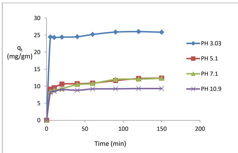
Figure 1: Effect of initial solution pH on the adsorption of CR onto pine leaves; adsorbent 15 mg, volume of dye solution 50 ml, initial dye concentration 10 ppm, temperature 30 °C, shaker speed 150 rpm.
