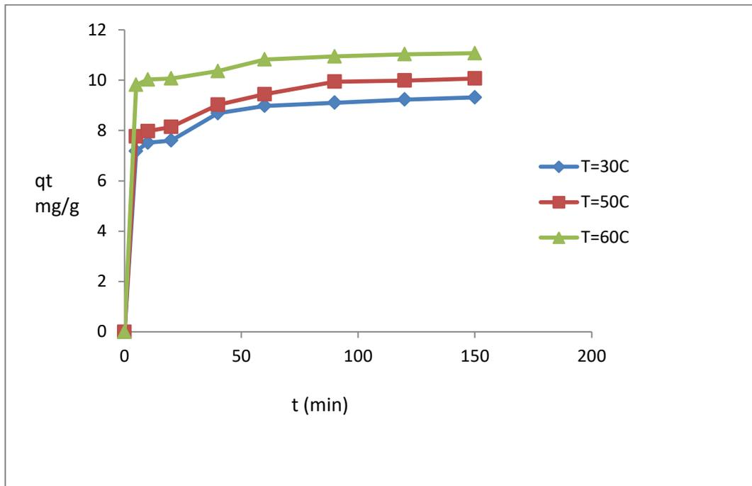
Figure. 3 Effect of temperature and time contact on the adsorption of CR onto raw pine leaves powder: Mass of Adsorbent 15 mg; Volume of CR Solution 50 ml; Initial CR Concentration 10 ppm; pH 6.25; Shaker Speed 150 rpm.
