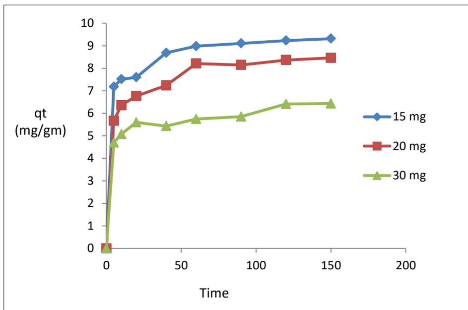
Figure 2 Effect of adsorbent dosages on the amount of CR adsorption by raw pine leaves biomass. Volume of CR Solution 50ml; Initial CR Concentration 10 ppm; pH 6.25; Temperature 30 °C; Shaker Speed 150 rpm.
