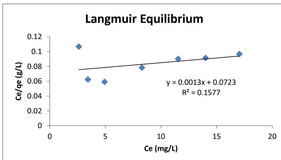
Figure 10 Langmuir plot: Amount of adsorbent (pine leaves) added 10 mg; Initial CR Concentration 10, 20, 30, 40, 50, 60, 70 ppm; pH 3.03 Temperature 30 oC; Shaker Speed 150 rpm.
