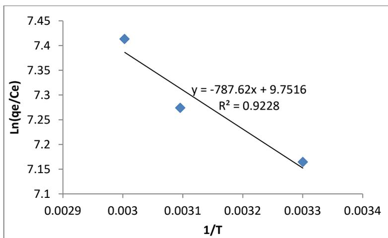
Figure 11: Study of Thermodynamic Properties for Adsorption
