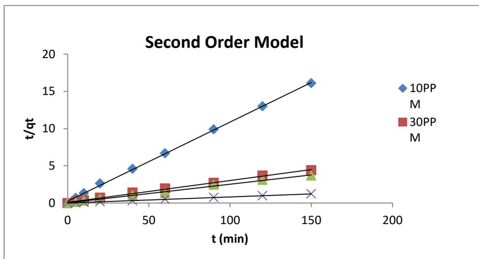
Figure 8: Pseudo-second-order kinetic model for CR adsorption at different initial solution concentration: Mass of Adsorbent = 15 mg; Volume of Dye Solution = 50 ml; pH = 6.25; Temperature = 30°C; Shaker Speed = 150 rpm
