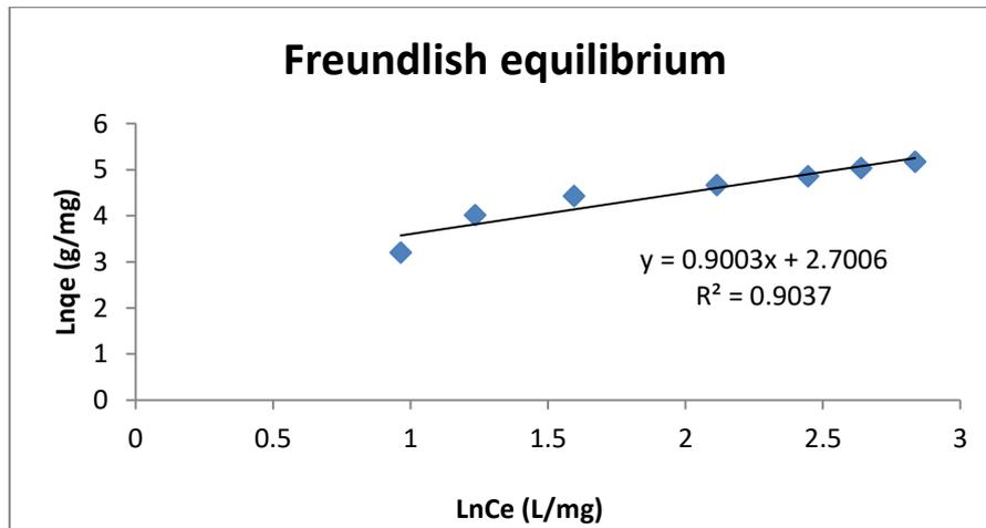
Figure 9: Freundlich plot: Amount of adsorbent (pine leaves) added 10 mg; Initial CR Concentration 10, 20, 30, 40, 50, 60, 70 ppm; pH 3.03 Temperature 30 oC; Shaker Speed 150 rpm.
