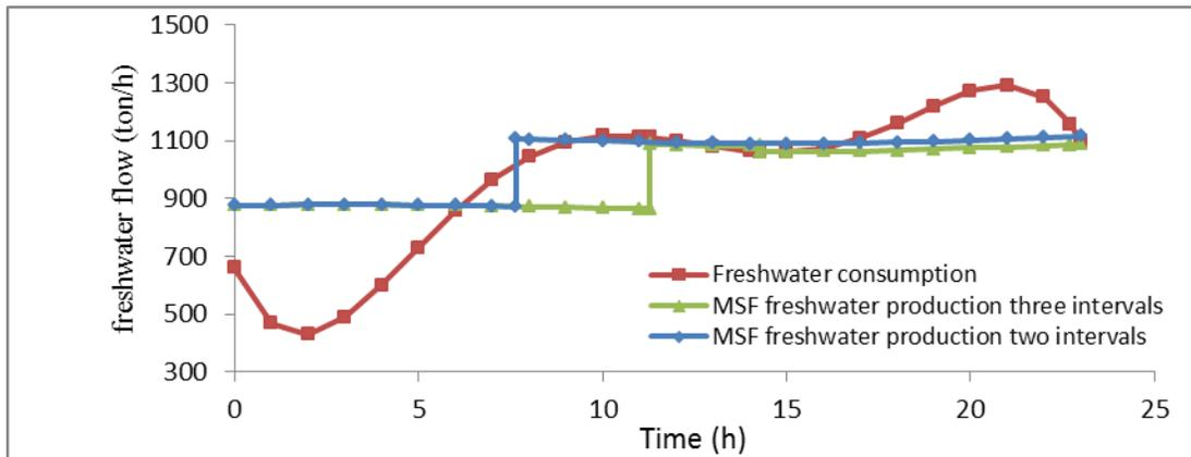
Figure 9 Freshwater consumption and production profile at different intervals
