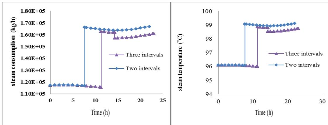
Figure 7 Changes in steam temperature and consumption profiles in two and three time intervals
