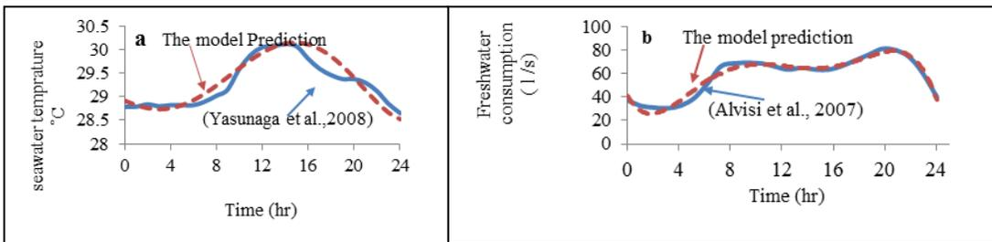
Figure 2 (a) Temperature of Seawater and (b) Fresh water demand/ consumption profiles[1]
