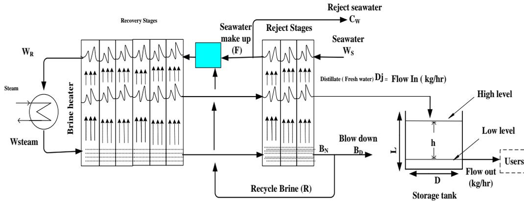
Figure 1 A typical MSF desalination process with storage tank [1]
