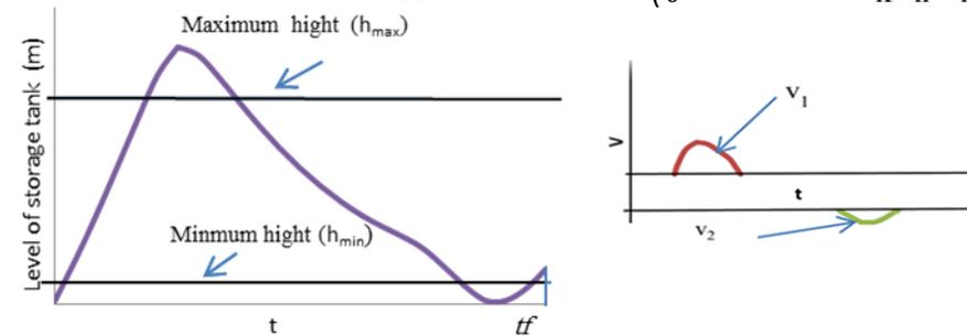
Figure 3 A typical storage tank level profiles
