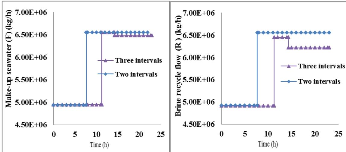
Figure 6 Optimal flowrate of seawater make up (F) and brine recycling rate (R) profiles in three and two time intervals
