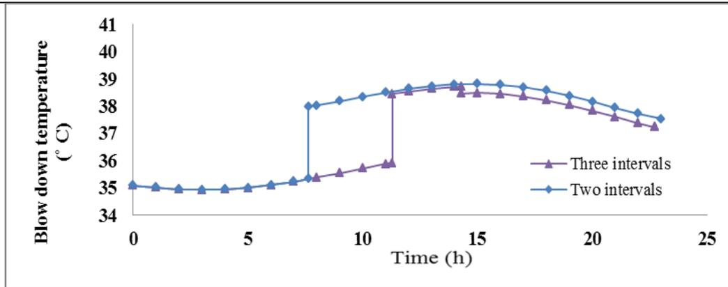
Figure 8 Variations of blowdown temperature profiles at three and two time intervals
