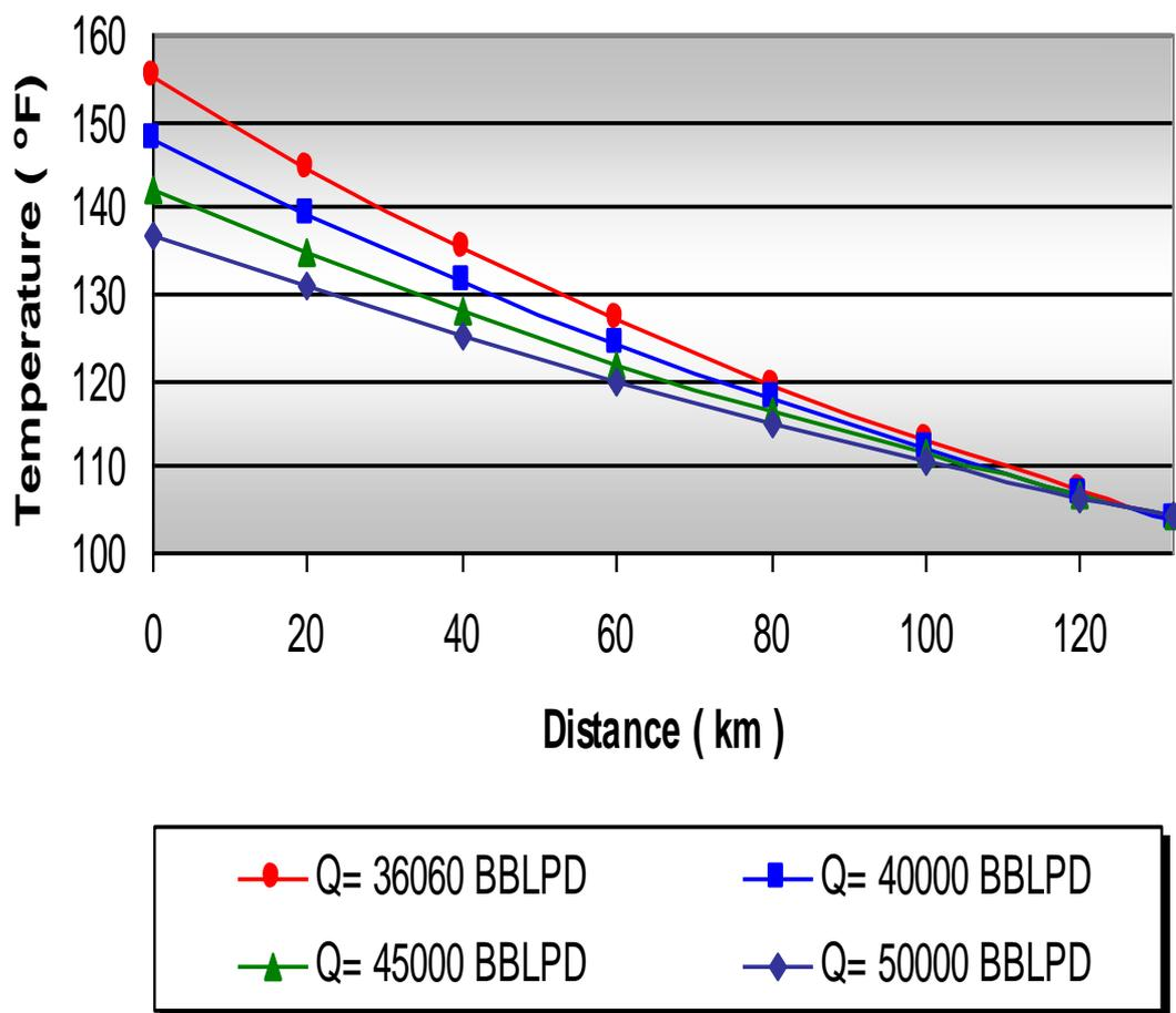
Figure 3: Temperature Profile for Constant Final Temperature.
