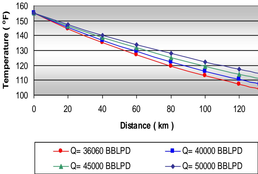
Figure 2: Temperature Profile at Constant Inlet Temperature.
