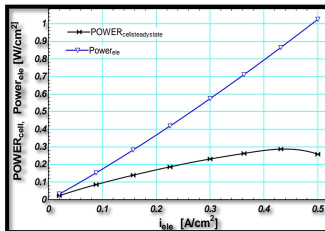
Fig. 5. The change in the power of alkaline electrolysis and PEM fuel cell by changing in current density.
