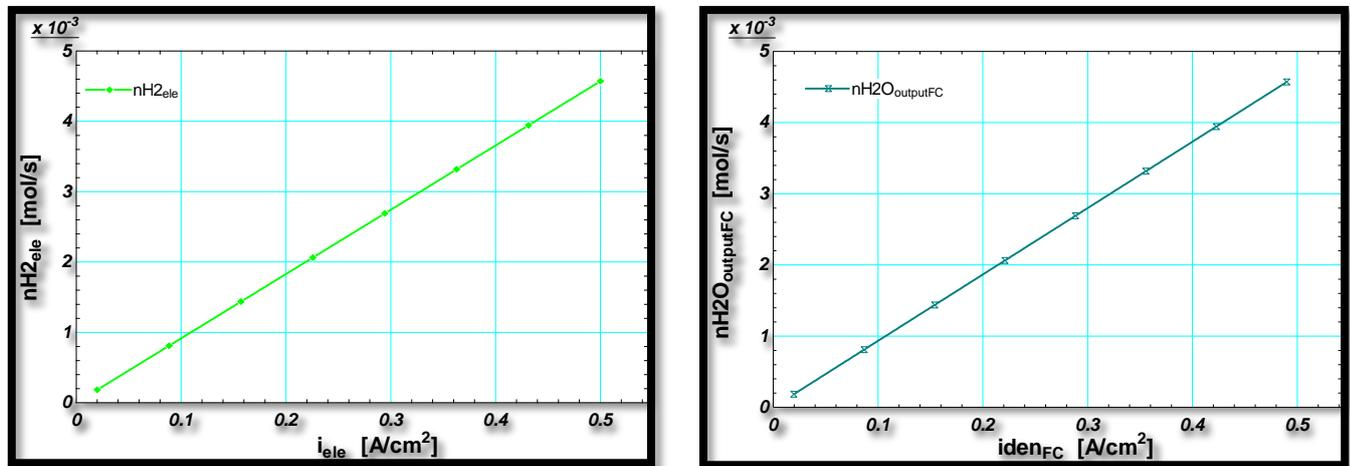
Fig. 4. The change in the Hydrogen production from the alkaline electrolysis and PEM fuel cell by changing in current density.
