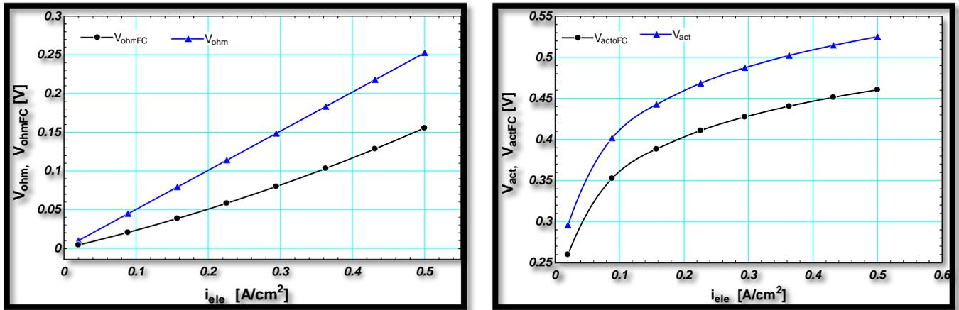
Fig. 3. The change in the activation and ohmic voltage of electrolysis and cell with change of electrolysis current.
