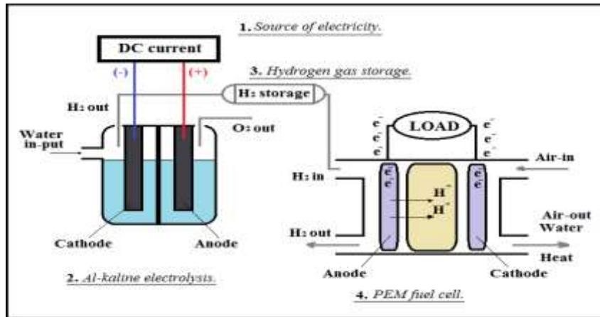
Fig. 1. Layout for DCS system.
