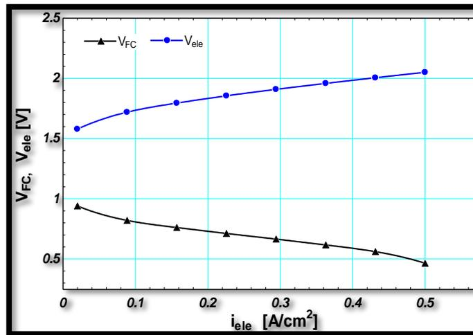
Fig. 2. The change in the voltage of alkaline electrolysis and PEM fuel cell by changing in current density.
